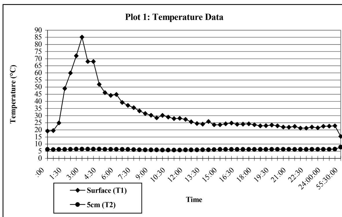
**Figure 9.** HH12 digital thermometer temperature data from surface and subsurface (5 cm) thermocouples placed in plot 1.
