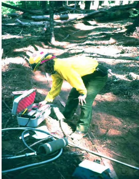
**Photograph 2.** Thermocouples were placed into the soil by the obsidian samples to monitor soil temperatures. A cable led from the thermocouples to a datalogger, located outside the fireline. The datalogger was set to record temperatures at the obsidian samples at designated time intervals.
